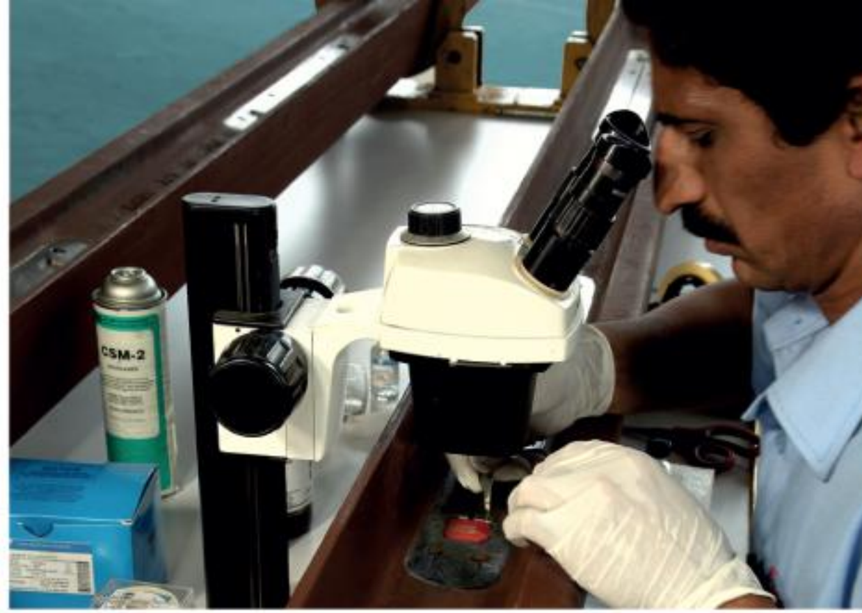
Precision bonding of strain gauges
